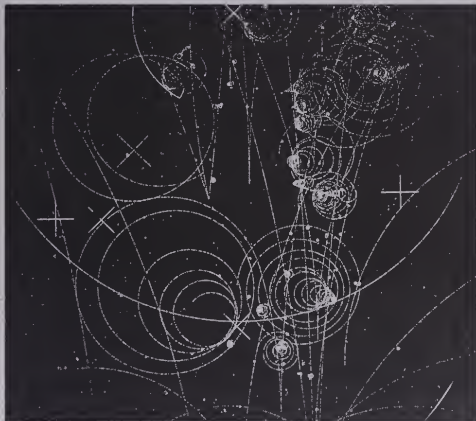
Bubble-chamber tracks. The tight spirals are mostly electrons; heavier particles swerve less in the magnetic field.
