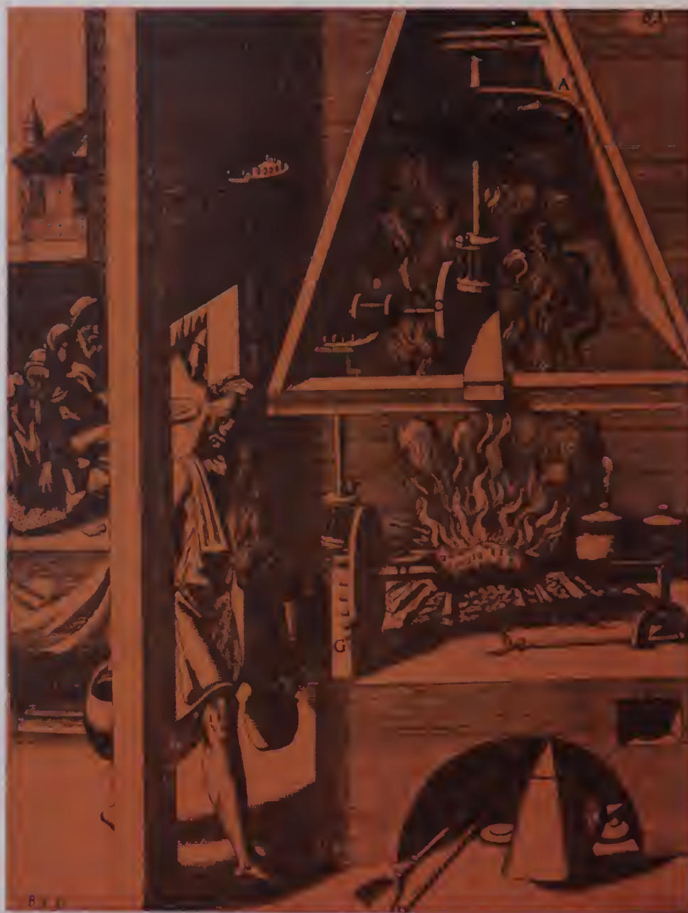
Above, the smoke-jack, from a book of 'new devices' published in 1662. Below, left, diagram of a Roman hypocaust or under-floor heating system. Below, right, a fragment of early 16th-century wallpaper, showing the royal crest.
