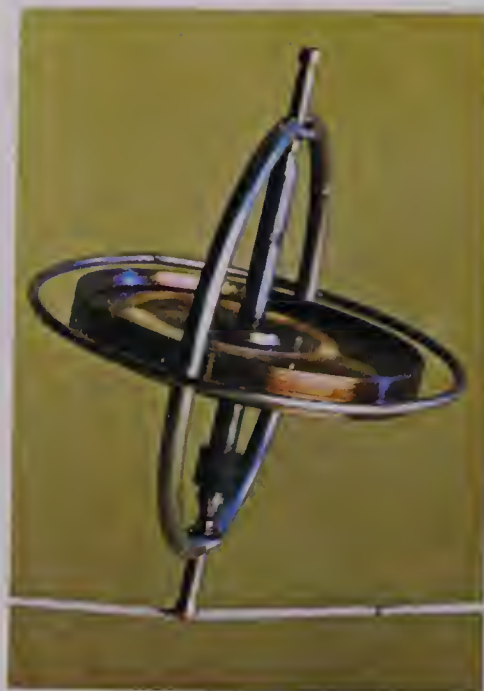
The gyroscope, the ultimate stable source of reference: essentially a simple device, yet it has many uses, from the stabilization of ships at sea to the control of blind flying in the air.
