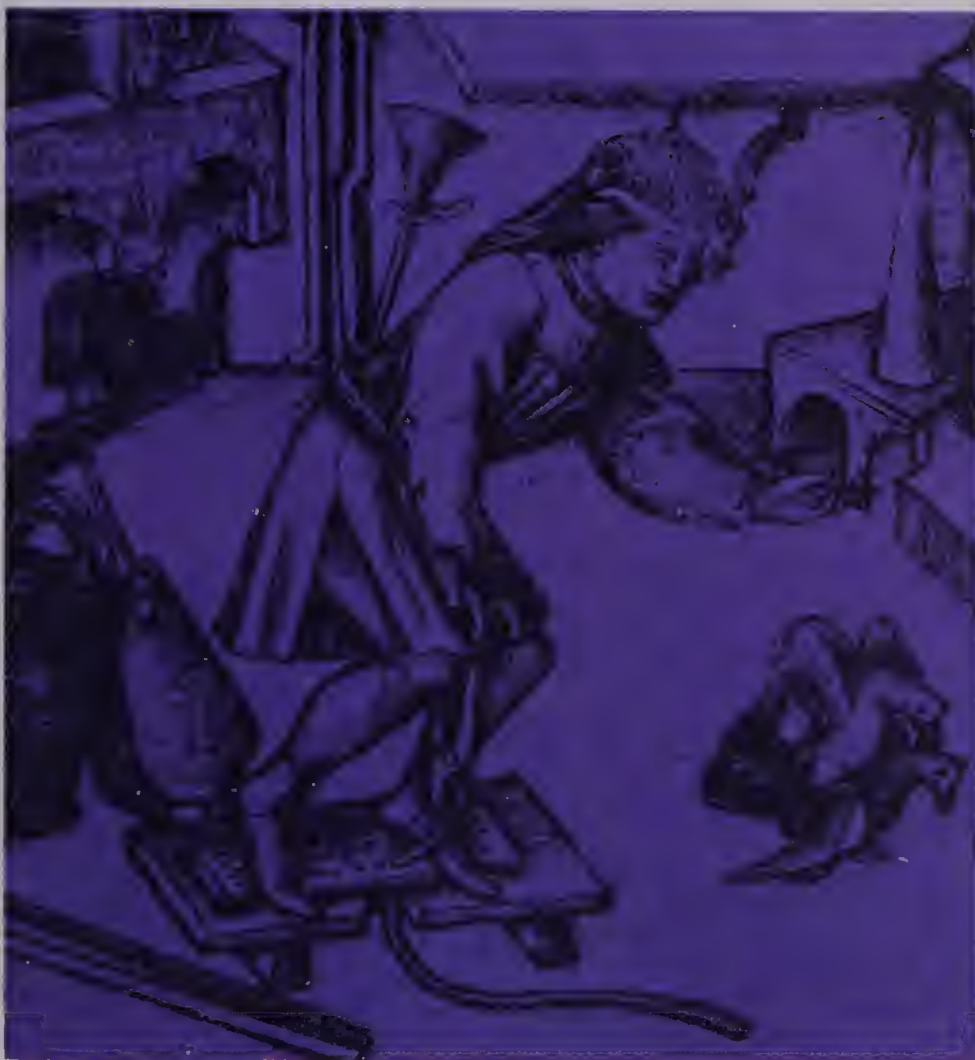
Detail from an etching, St Eligius in the Goldsmith's Shop, by the Master of Bileam. Drawing the wire through the dies by hand must have needed both strength and control.
