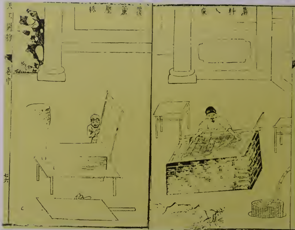
Above, paper-making in 17th-century China. On the left, a sheet of wet pulp is placed under a wire screen for pressing. On the right, the pressed sheets of pulp are laid on an oven for drying.
