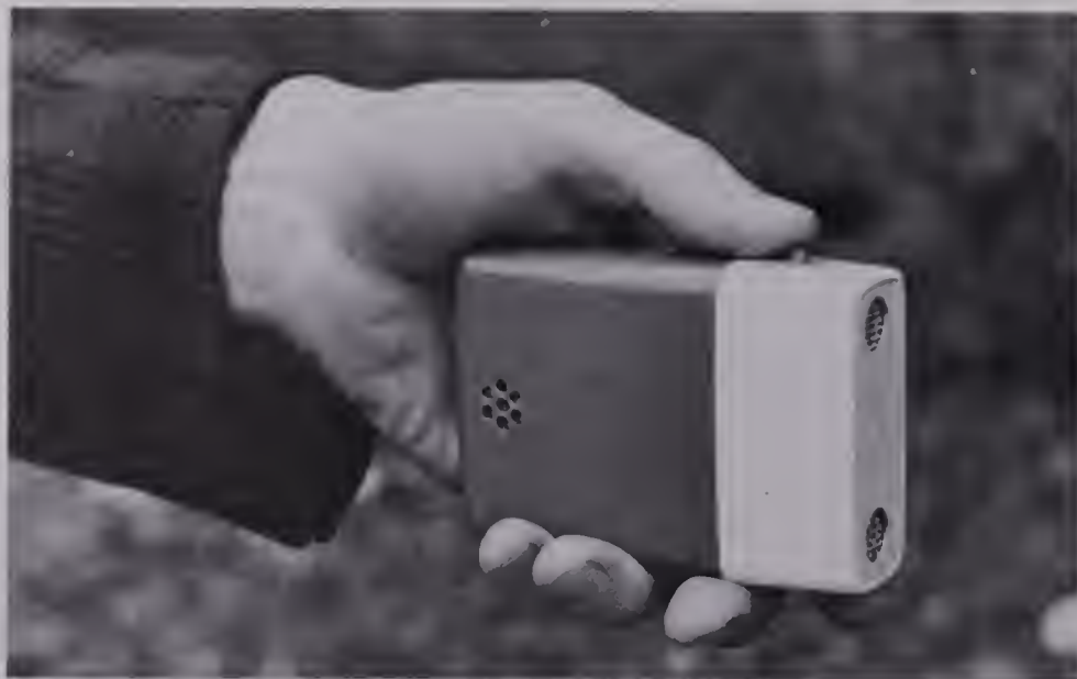
An experimental ultrasonic aid for the blind. Sound waves reflected back from an obstacle are transformed into an audible 'beep' in a small receiver or into a buzz that can be felt in the hand.
