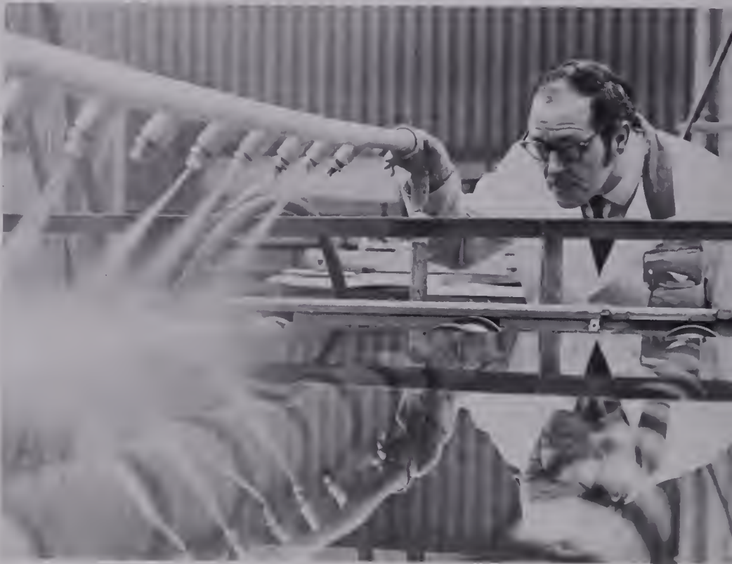
Below, continuous ribbon of float glass, 4 mm. thick. The reflection suggests the perfect flatness produced by this method.
