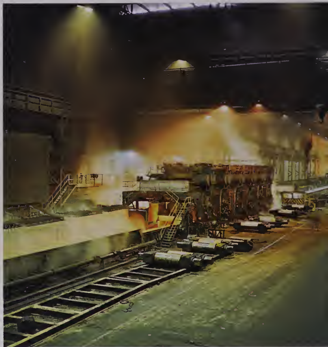
Automation in a steelworks: six-stand hot finishing mill at British Steel's Llanwren works. The process is computer-controlled and entirely automatic.
