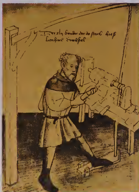
Medieval pole lathe, worked with the foot. By its aid, such things as table legs were considerably easier to make.
