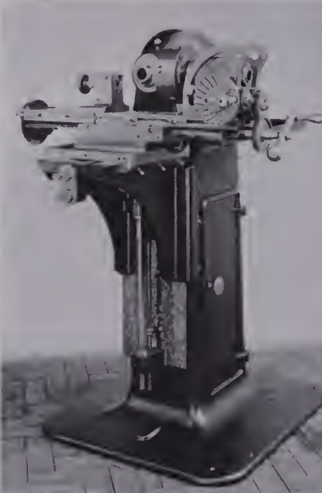
The 'universal' milling machine, invented by Joseph R. Brown and shown at the Paris Exhibition of 1867.
