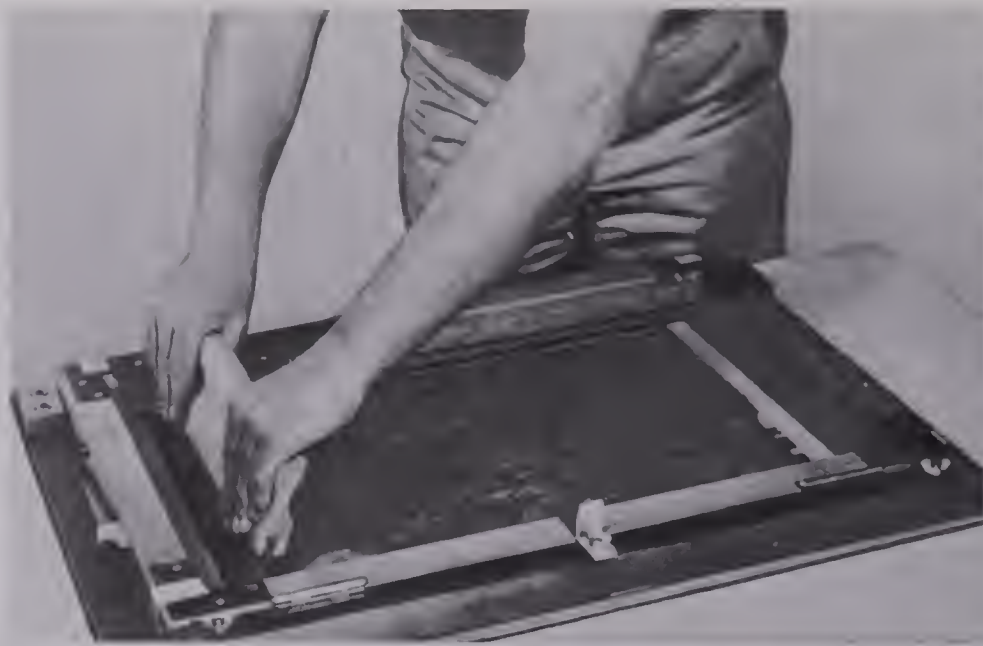
Silk-screen printing: spreading the colour with the 'squeegee'.
