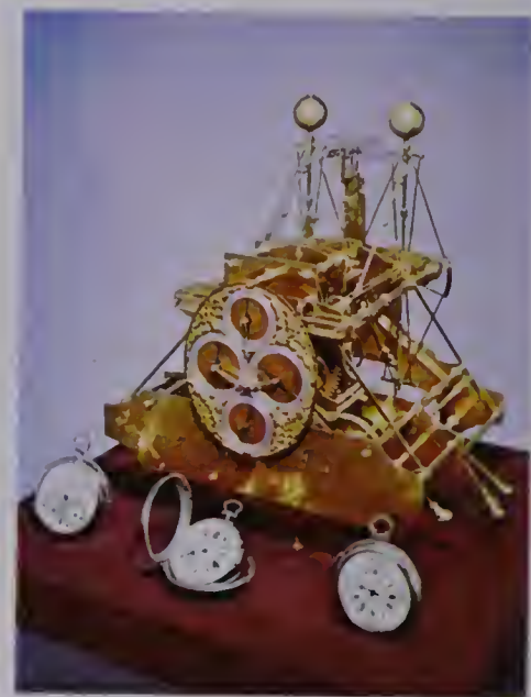
Harrison's first marine chronometer, made in 1735, with smaller versions, including (foreground) Kendall's duplicate taken by Cook on his second voyage.
