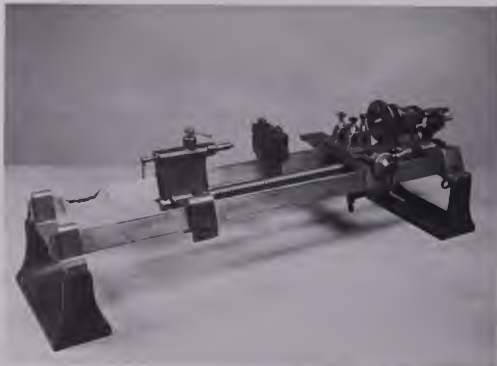
Henry Maudslay's original screw-cutting lathe, invented in 1800.
