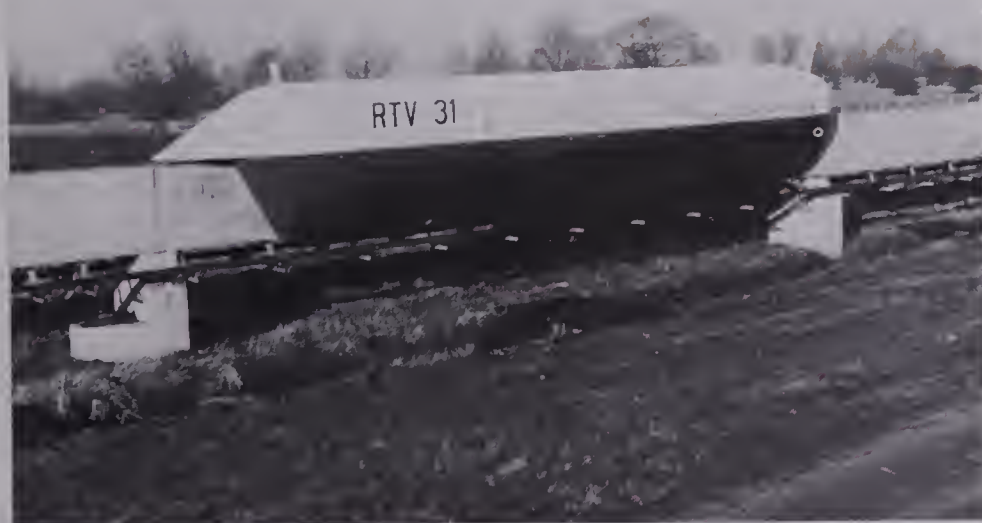
Above, experimental tracked hovercraft. Propelled by a linear motor (q.v.), it has a design top speed of 300 m.p.h.
