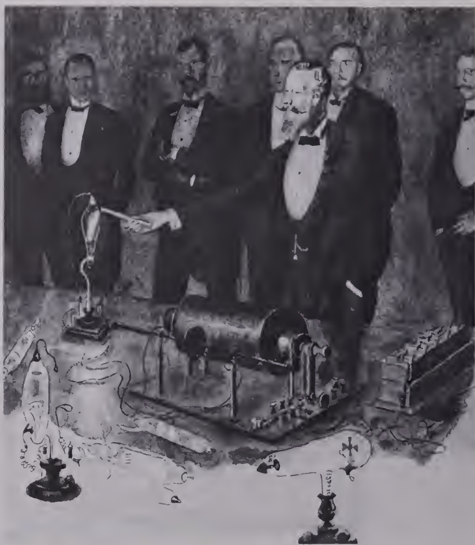
William Crookes demonstrates the deflection of cathode rays by a magnet.
