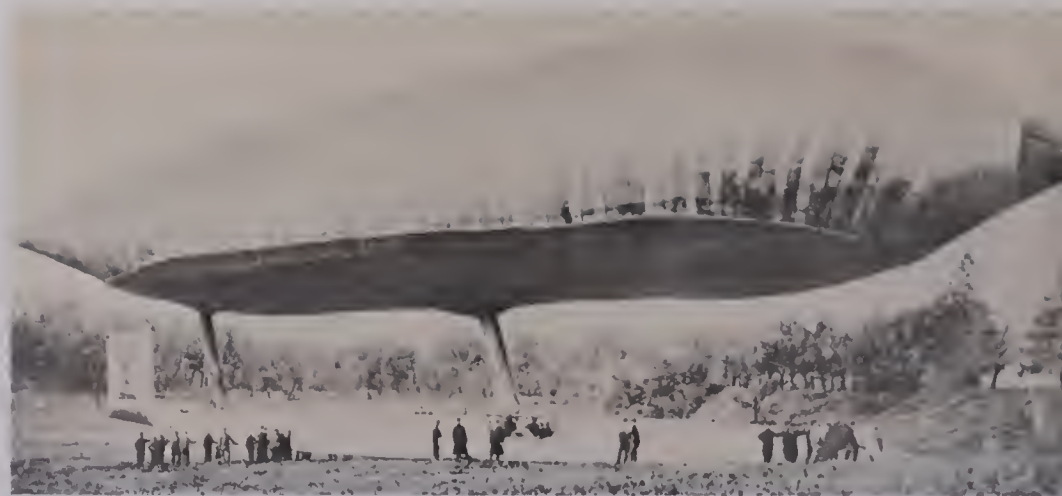
La France, designed and built by two French Army officers, was the first airship sufficiently fast to follow her pilot's directions – on a calm day. Her pioneer flight of some five miles took place in August 1884.
