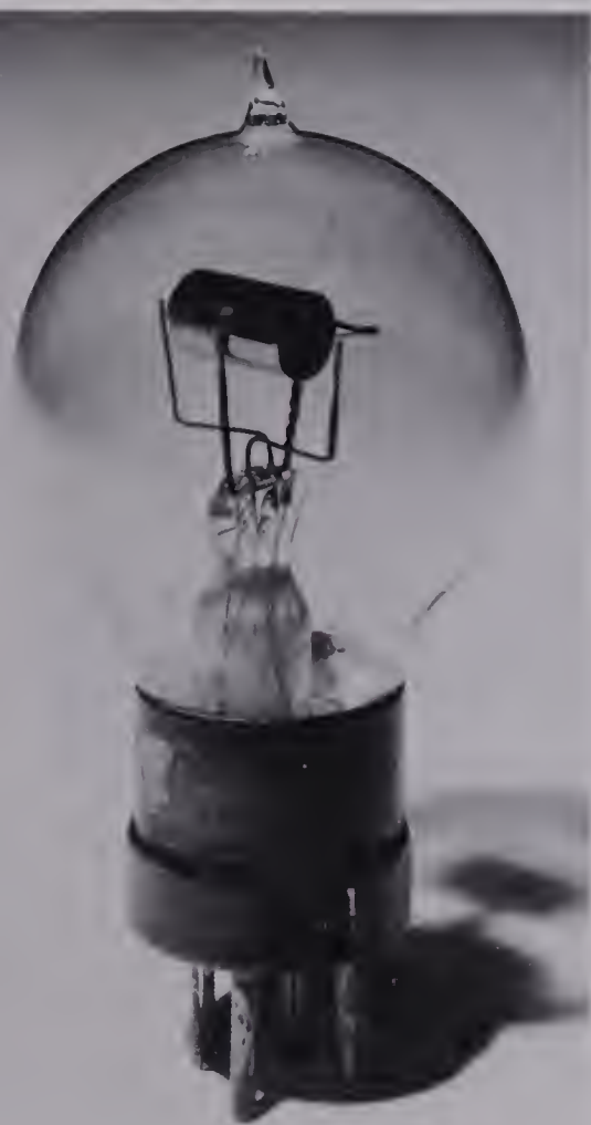
Fotos Type R triode. Without this modulating device, sound transmission would have been impossible, either by wire or by radio.
