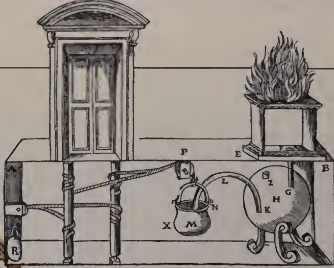
Hero of Alexandria's device for opening a door with fire
