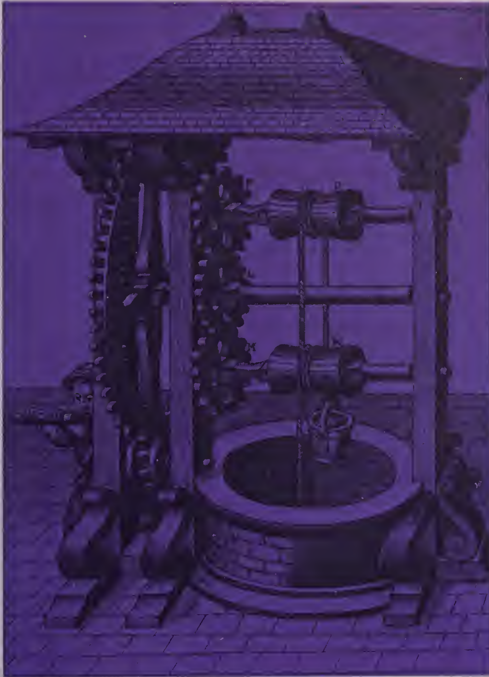
Gears would have made easier the turning of this outsize well-handle. From Agostino Ramelli's Machine, 1588.
