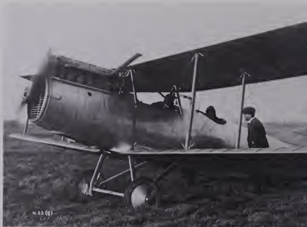
The Short 'Silver Streak' one of the first aircraft with 'stressed skin' construction.
