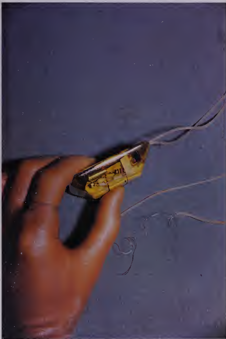
A modern cardiac pacemaker. First seriously suggested in 1862, the first working model, made 70 years later, weighed 7.2 kg.
