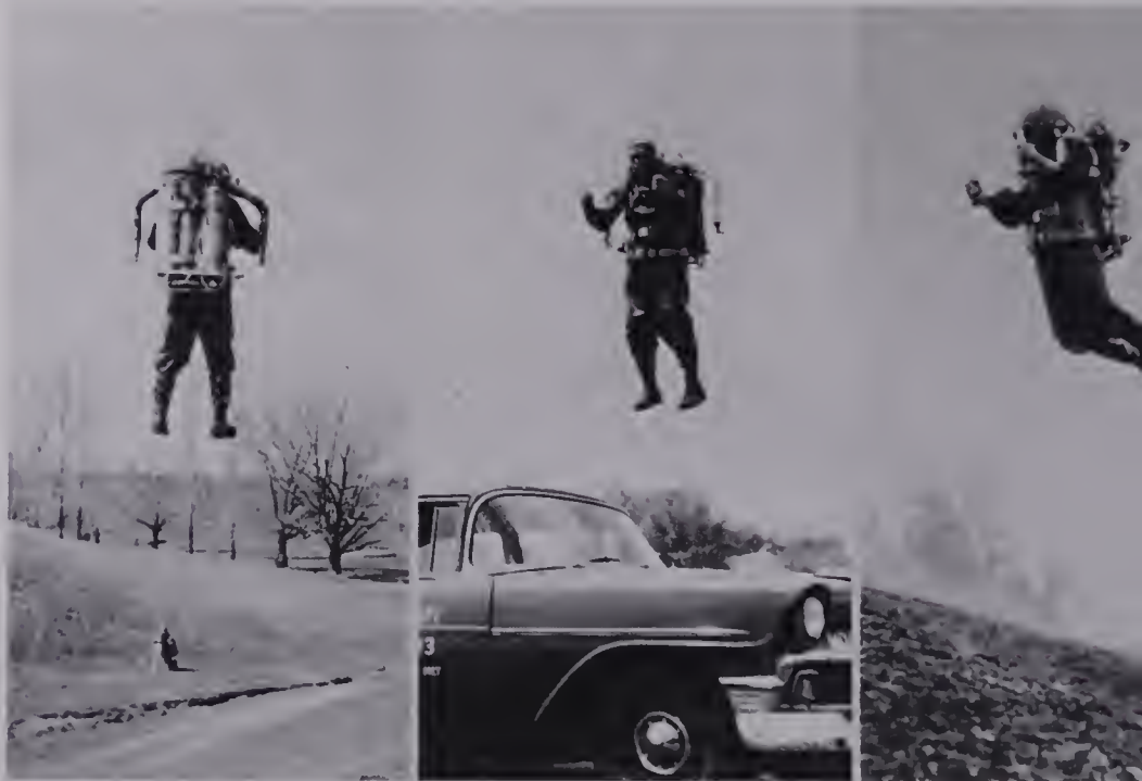
The Bell Aerosystems rocket belt, powered with hydrogen peroxide, has hand throttles for control of thrust and for steering.
