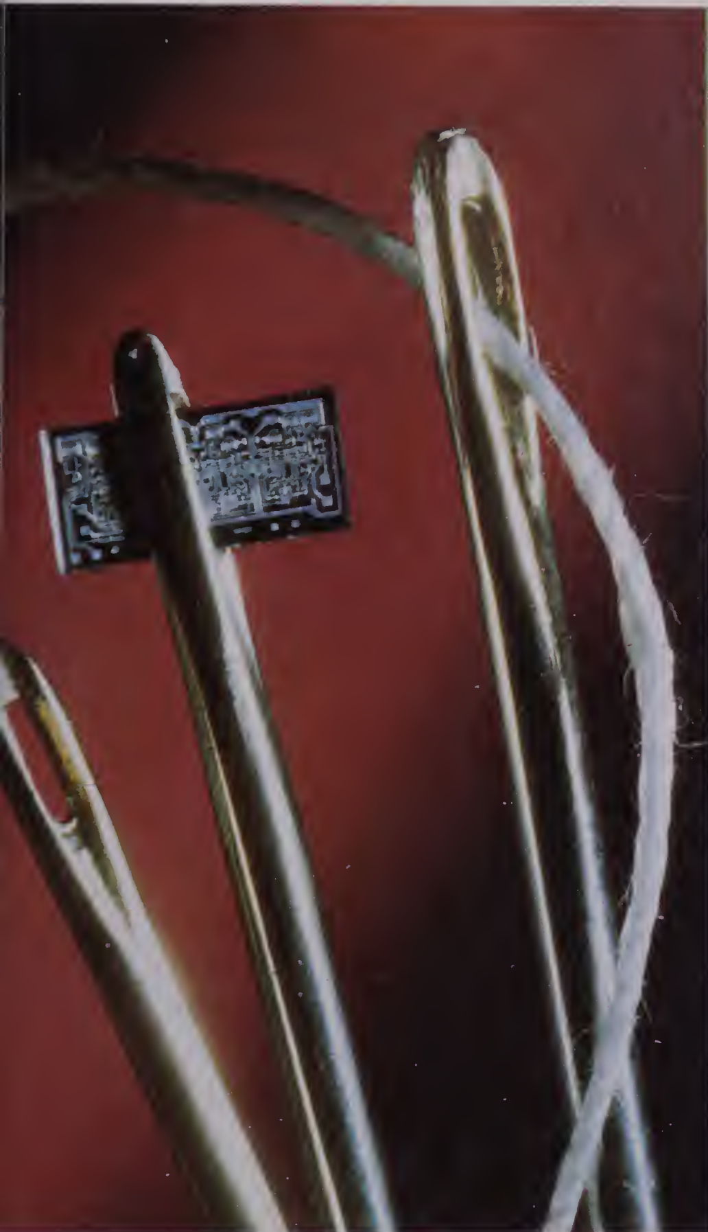
Before encapsulation in plastic, this tiny silicon chip with its complex printed circuit and over 120 components can pass through the eye of a needle. Such micro-miniaturization has only become possible with the invention of the transistor.
