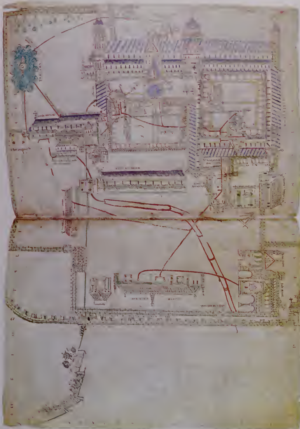
Plan of the Benedictine Monastery of Christchurch, Canterbury, showing the projected water-supply and drainage system, c. 1160.
