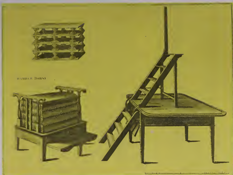
This design by Thomas Sheraton (1793) for a 'chamber horse' shows in detail one of the first examples of springs in upholstery.
